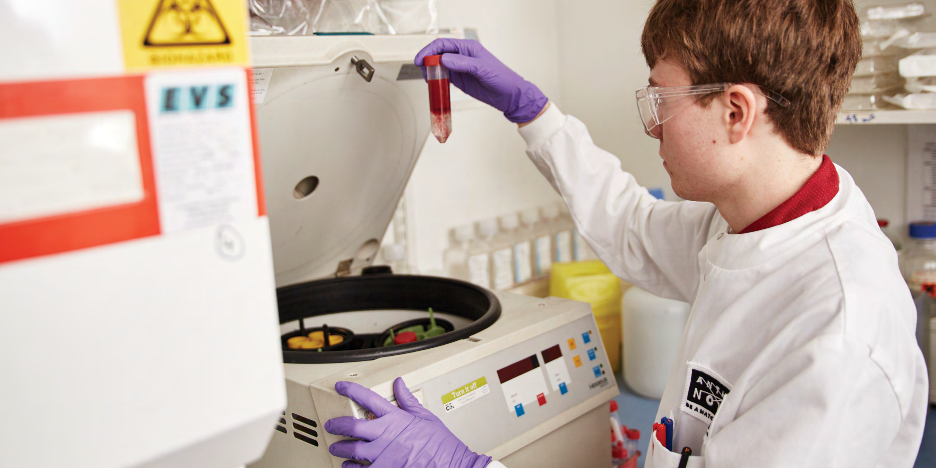
Above: Whole blood is layered onto lymphoprep solution and placed into centrifuge. After a 30 minute spin the blood will segregate into layers of red blood cells, lymphoprep solution, white blood cells and plasma.
