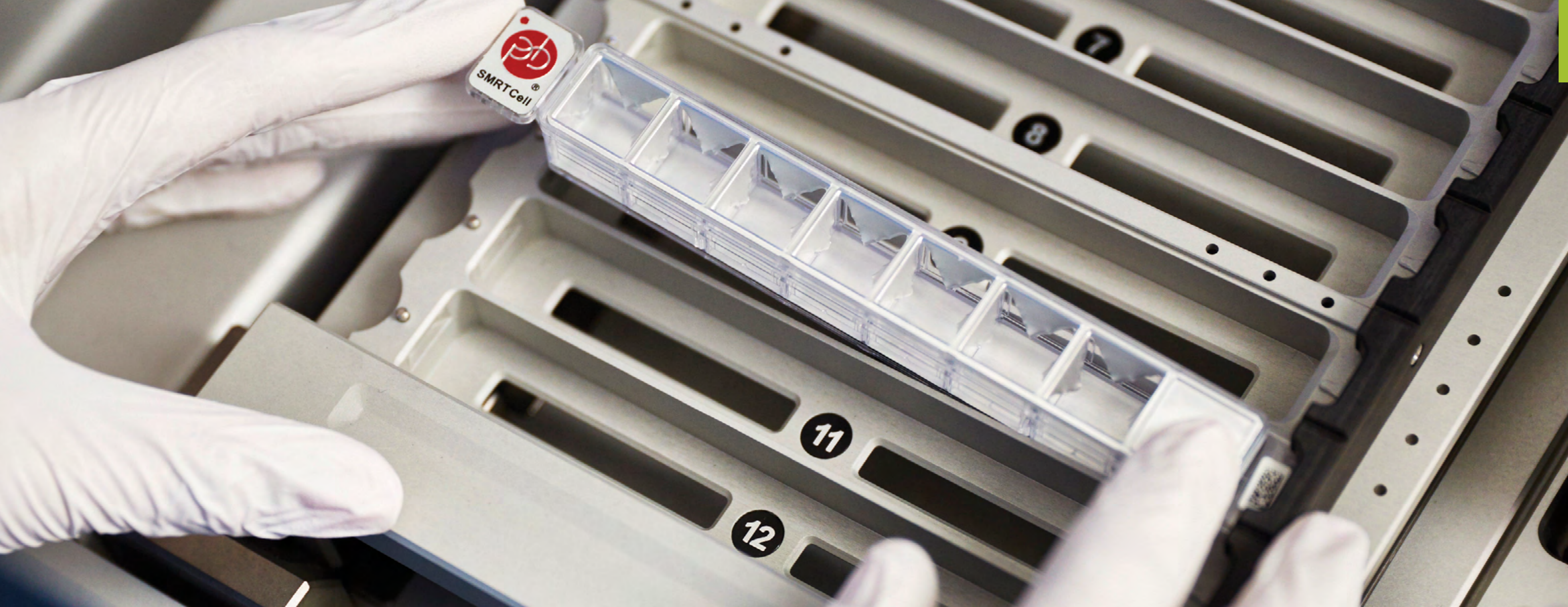
Above: A SMRTcell strip is loaded onto the PacBio-RS-II DNA sequencer. One SMRTcell contains 144 different genes from 48 people to be sequenced.
